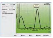
The GemsView configuration software can be downloaded free of charge. All user-modifiable parameters of the RLI-G can be set and all values can be queried through GemsView. Other features are: continuous "echo-map" reading, trend monitoring, data logging, data saving.
